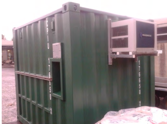
Mobile laboratory in a shipping container
